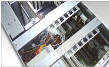
Two Adjustable Card Retainer Positions For fixing all the cards more flexibly and tightly
